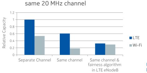
Capacity with LTE & Wi-Fi on the
