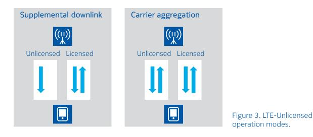
When operating with downlink only on the unlicensed band (supplemental downlink), the LTE eNodeB can perform most of the necessary operations to ensure reliable communications, including checking whether the intended unlicensed channel is free from other use.
